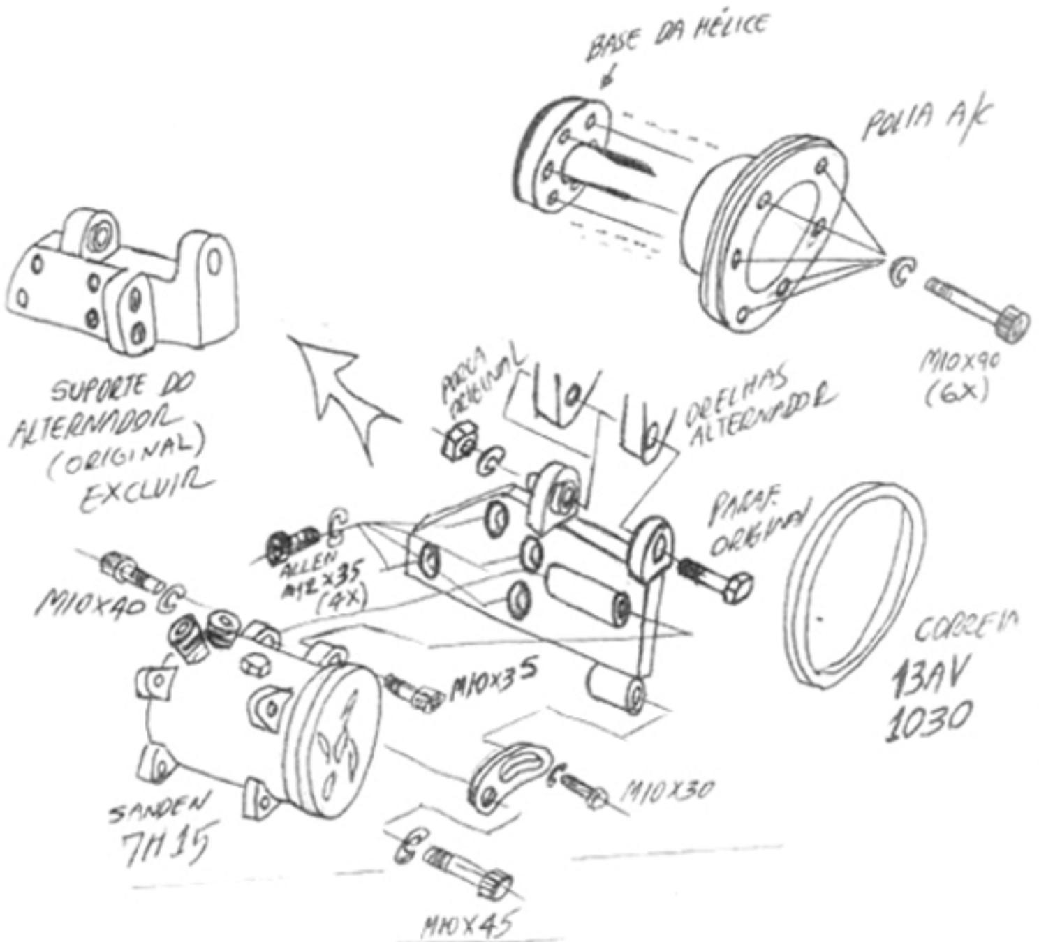
IMPORTANTE: INDISPENSÁVEL A TROCA DAS PASTILHAS QUE PRENDEM O SUPORTE DO COMPRESSOR E ALTERNADOR NO BLOCO DO MOTOR
